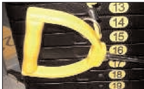
Right: A weight pin grip is large and open. The weight number labels are large, raised, and yellow (high contrast)
