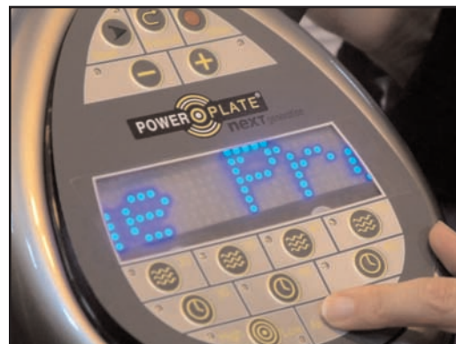
Right: An input console has tactile indicators to help users program exercise bicycles, steppers, treadmills, etc. The display uses large print.
